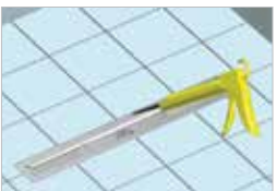
Fix the metal sash with silicon or joint.
