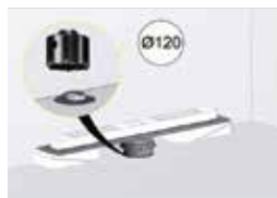
Drill the concrete with the help of drilling core for the pipe connection.
