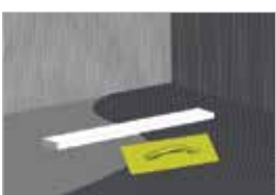
Spread the ceramic adhesive to the surface.
