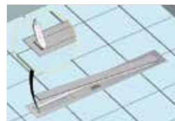
Clean the siphon with the help of cover key.
