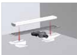
Place the insulation-finish metal case to the adjusting set.
