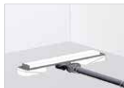
Connect the shower channel to the installation and put the protective styropor in case of blockage.
